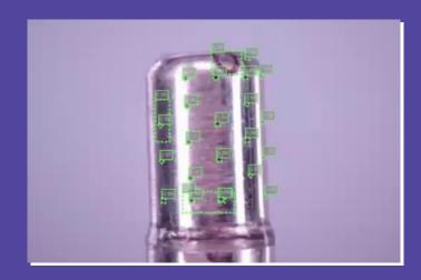
An Al vision system inspection image of a catheter tip, assessing the placement and integrity of the required holes.
